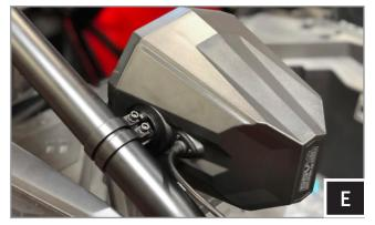
E. Route the speaker wire away from any moving parts and any sharp metal, then connect to the amplifier.
