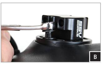
B. Loosely install the clamp base to the US-C68 with (2) M6x1.0x20mm screws and washers using a 8mm open-ended wrench. Position the clamp base to your desired position and tighten the (2) M6x1.0x20mm screws.
