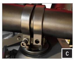
C. Wrap a plastic bag around the roll cage to prevent scratching. Press the clamps onto the roll cage over the plastic bag. Place the (2) M6x1.0x45mm screws and washers through the clamp and clamp base. Secure the clamps to the roll cage with a 5mm allen key.
