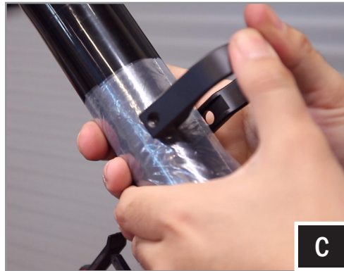
C. Place both ring mounting clamps on the cage using the plastic bag to prevent scratching, place the cage mount pod in its final mounting location and secure to the clamps using the two (2) M6 allen socket head bolts and washers with a 5mm allen key.
