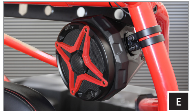
E. Route the speaker wire away from any moving parts and any sharp metal, then connect to the amplifier.
