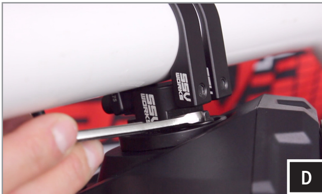
D. Position the speaker to your liking and tighten the hex head bolts by hand with a 8mm wrench.
