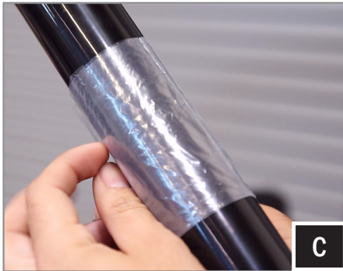
C. Place both ring mounting clamps on the cage using the plastic bag to prevent scratching, place the cage mount pod in its final mounting location and secure to the clamps using the two (2) M6 allen socket head bolts and washers with a 5mm allen key.
