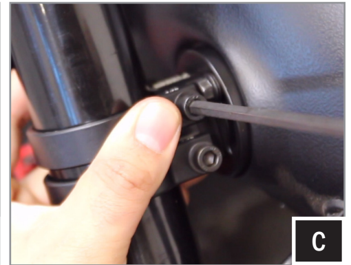
C. Place both ring mounting clamps on the cage using the plastic bag to prevent scratching, place the cage mount pod in its final mounting location and secure to the clamps using the two (2) M6 allen socket head bolts and washers with a 5mm allen key.
