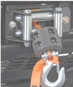
The winch stop is universally designed to fit steel or synthetic cables up to 1/2" diameter. *Note, installation may be easier if certain items are removed from vehicle first.*
